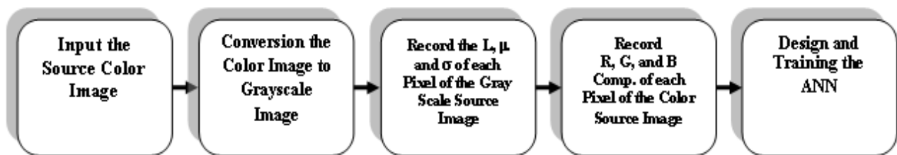
Figure 1: A Simplified Block Diagram of the First Phase of the Proposed Technique
